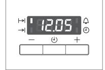
When the time has elapsed, the function indicator flashes, an audible signal sounds for 2 minutes and the oven switches itself off.
